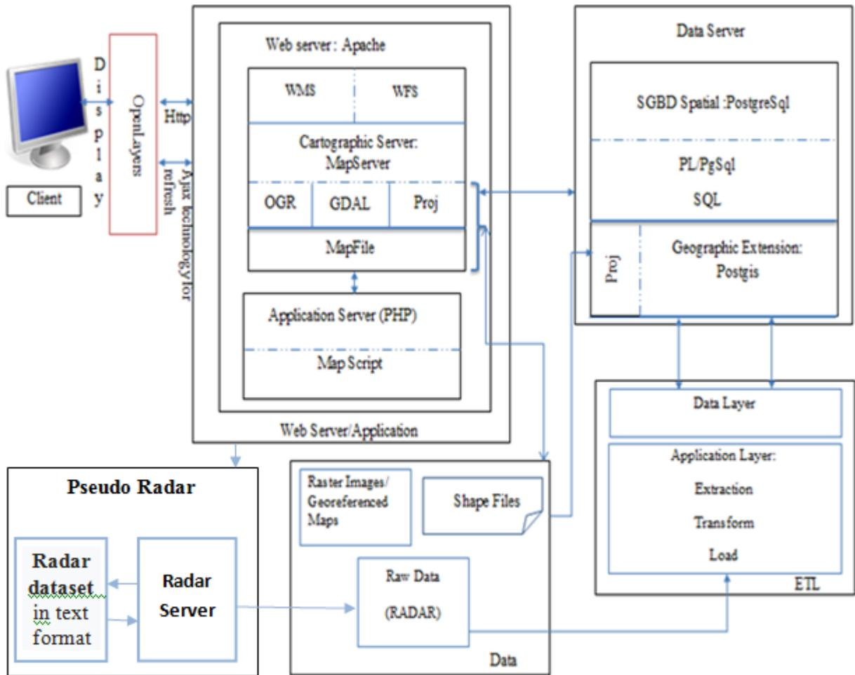
**Figure 3:** Architecture of the Proposed Solution
