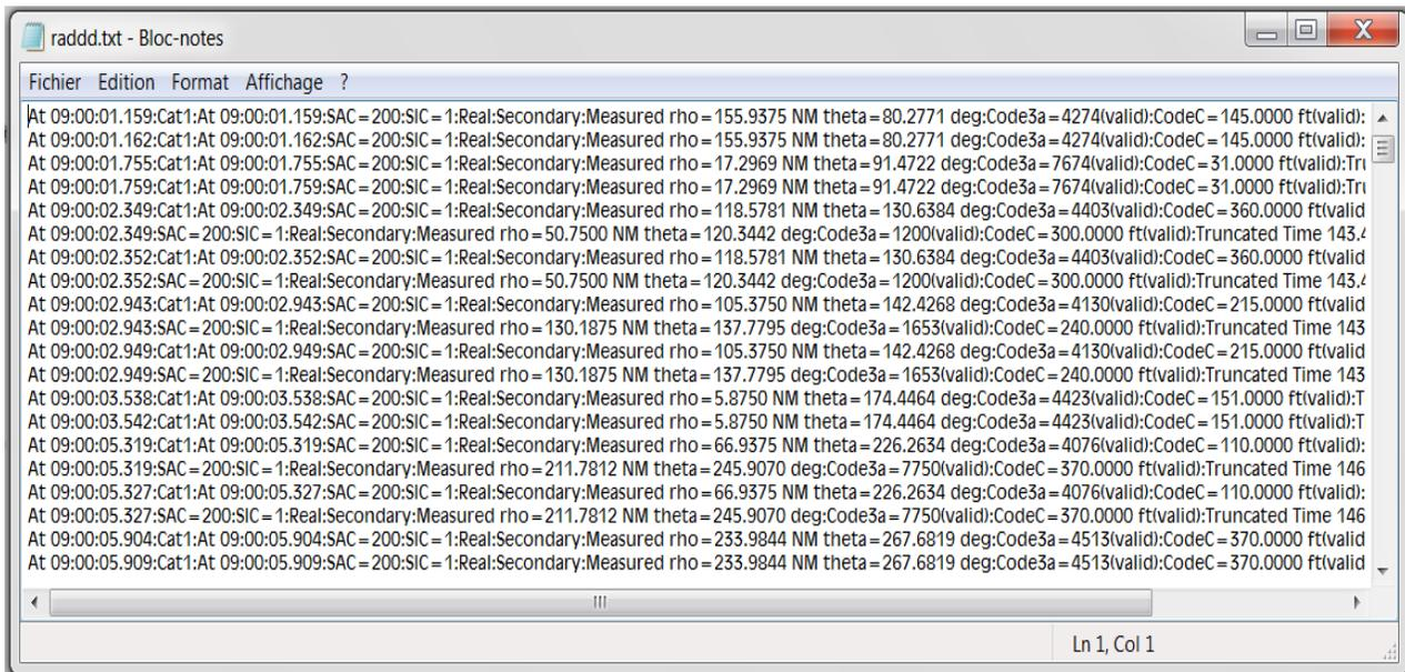
**Figure 2: Sample Radar Data in ASTERIX Format saved in a File and Displayed in Clear Text**
