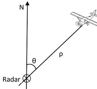
**Figure 1:** Positioning of the Aircraft in Relation to the ATC Radar
