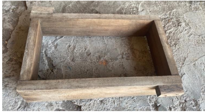
Figure 1: Wooden mold measuring 5.5 x 14 x 25.5 cm
